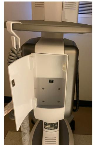
**4.2** Connect the stethoscope into the USB port which is located on the expansion panel.
